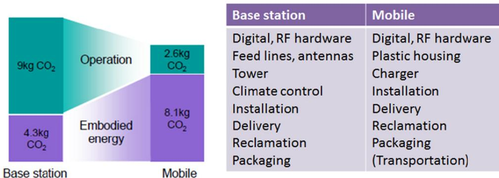
**Figure 8.** Operational and embodied energy for a base station and mobile unit for cellular wireless communications [9]. The embodied energy is a relatively larger portion of the total energy consumption of a mobile unit because the operational energy is significantly lower than in the base-station case (<1W of radiated power, compared to >100W).
