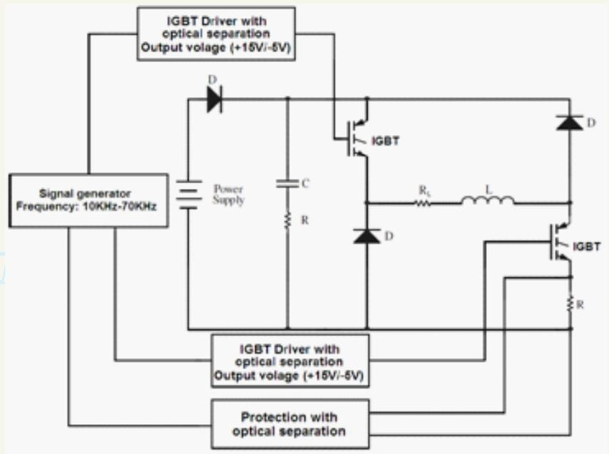
**Fig. 6.** Block diagram of the Chopper circuit.
