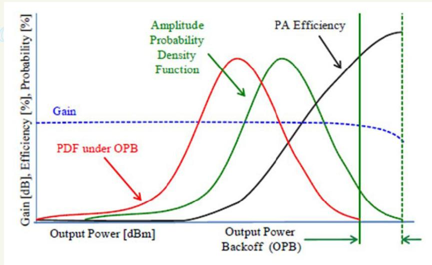
**Figure 7.** Typical PA efficiency and gain behavior over output power. Probability density functions for a high-PAR signal at two average output power levels are overlaid.
