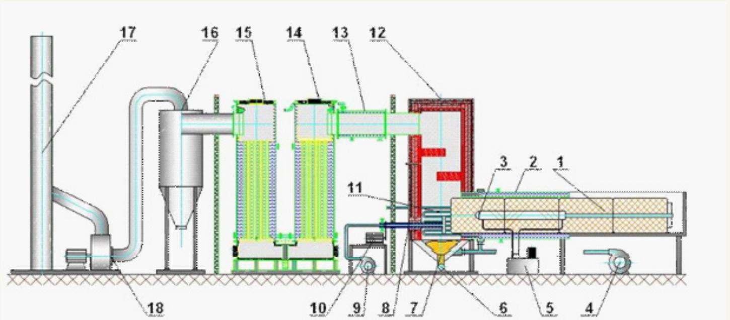
**Figure 7** Scheme of the hot-water industrial boiler, power 1.5 - 2 MW
