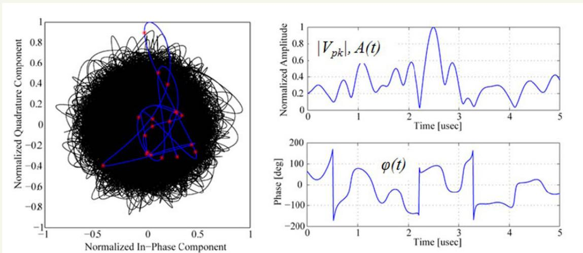
**Figure 6.** Polar plot (left) and time-domain plot of amplitude and phase (right) of a W-CDMA cell-phone signal shows very large swings in amplitude which happen extremely quickly.
