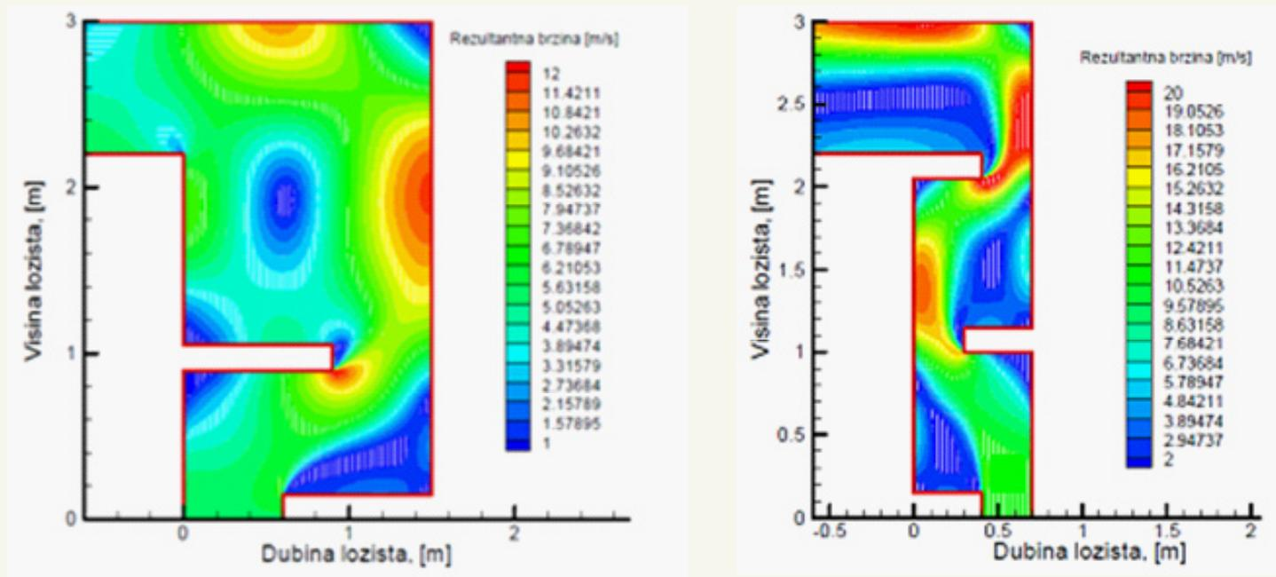
Figure 5 Profiles of the flue gases velocities in two versions of the adiabatic furnace
