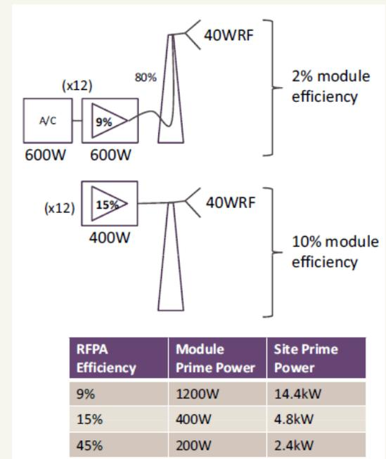
**Figure 5.** Example approximate power consumption of a 9% efficient 40-W radio-frequency PA module (older design), a 15% efficiency PA (current designs) and a future 45% efficient PA. The difference in prime power consumption is almost a factor of seven.
